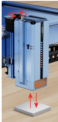
40W fixed focus, focal length 8mm
